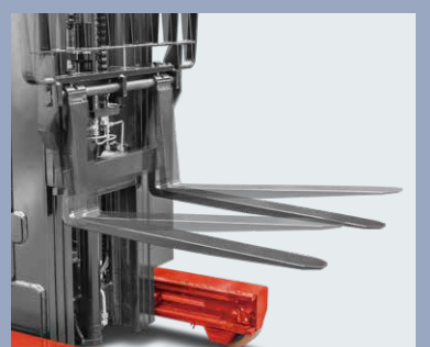
Forks can tilt forward/backward for easy loading
