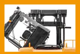
The over-turnable cab and electric tipping cylinde make tipping easier and more labor-saving.
