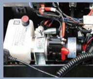
Integrated hydraulic unit, compact structure less space
