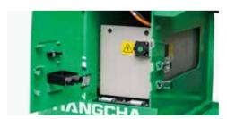
The side movable battery is equipped for standard configuration, which are convenient for battery replacement and repair.
