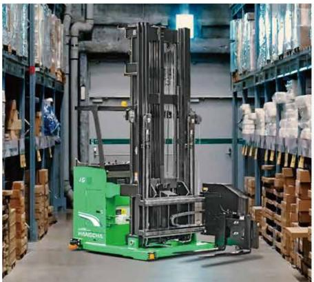
The adoption of mature mechanical disc brake allows emergency stop and parking, highly reliable.
