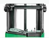
The new design of the mast structure enables the stacker to have an excellent operating view and to access the pallet more easily.
