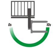
**Pivot Speed** Complete a full, 180-degree pivot in 10 seconds.
