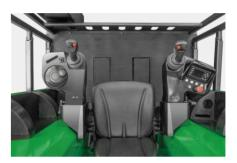
The double safety pedals, left and right guardrails, automatic induction joystick and other active and passive safety systems are equipped to prevent hazards caused by mis-operation.
