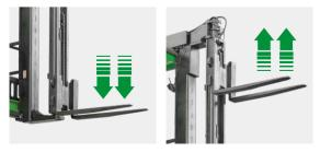
Equipped with the electro-hydraulic control buffer system, the fork slows down automatically when arriving at an end of any position to reduce the impact.
