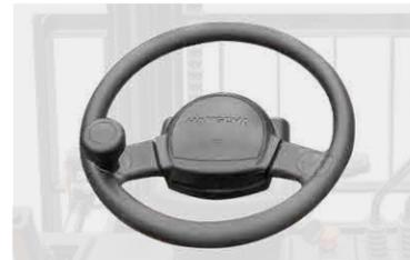
Large diameter steering wheel for flexible steering and more effortless operation.
