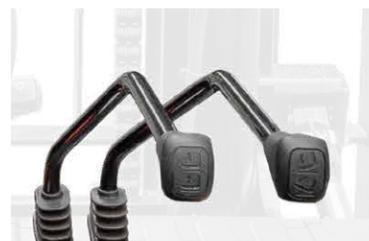
Increase the lever ratio to the control lever, resulting in less control force and more comfort.
