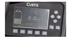
The large-screen anti-glare LCD display adopted can display power, speed, mileage, fault and other information clearly and accurately even in harsh environments.
