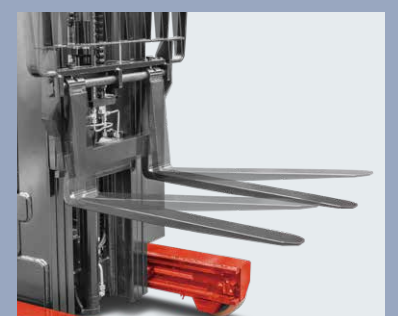
Forks can tilt forward/backward for easy loading
