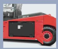
A series features battery side roll out as standard
