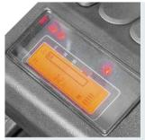
Newly-developed LCD instrument has more comprehensive functions and more stable performance and entirely displays the full truck state, fault code and other important information, which can make the operator more intuitively and conveniently have a better knowledge of truck state and make the maintenance conveniently.
