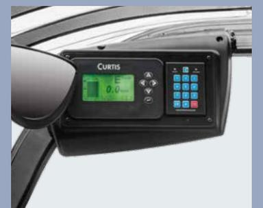
Easy to see dashboard is relocated to overhead, no restriction of the operator's visibility. The forklift is also applied PIN code access for better management.
