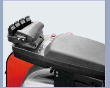
A series of high-performance version equipped with fingertip control on seat armrest, which can be four positions adjusted to meet different operator's demands, release operator fatigue. Emergency switch, horn, fingertip control levers are all centralized on the armrest, which via CAN bus connection, provide good reliability.
