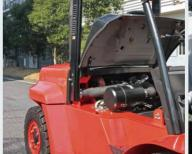
The enlarged opening angle of hood and increase of left and right hood side plates can provide you with convenient and rapid maintenance mode.
