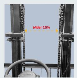
Adopt the new-type of box iron. Increase the inside width of inner mast and the spacing between lifting cylinders. The lowering of instruments in the driving cab will greatly increase the forward visibility; The rear visibility will also be greatly improved through the optimization design of counterweight.
