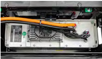
(Option)Lithium battery with the on-board charger(48V,20A) (Excluding model F2)
