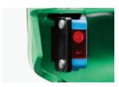
Foot detection sensor - trucks slows down or stops if operator's foot is detected outside of the platform contours (Rider model option).
