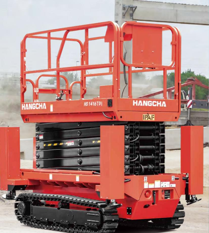
The scissor cylinder adopts proportional descent control, the moving speed changes gradually with the tilt angle of the operating joystick, and the descent is smooth and comfortable.
