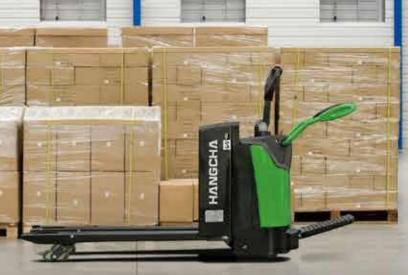
With AC walking motor, it has excellent acceleration performance, good climbing performance, low heat generation, no carbon brush and is maintenance-free.
