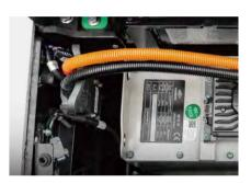
The power plug is fixed on the truck body to avoid damage from battery installment.
