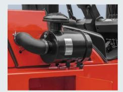
Optimized air intake and exhaust system of full vehicle, high-capacity exhaust silencer will reduce the noise of full vehicle and reduce the vibration.
